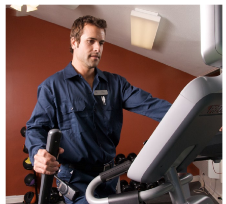
To begin testing the Cross Trainer, turn the machine on by getting on it and start stepping slowly.
