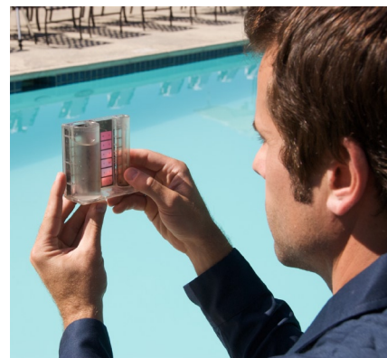
Pool water pH and Chlorine-Bromine levels must be tested three times a day and recorded.
